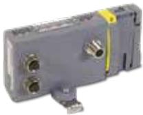
The P2M Industrial Ethernet 24 DO node offers 2 Ethernet ports allowing a line topology without external switch. The Ring topology can also be supported (enable/disable) for Profinet, EtherNet/IP and Modbus TCP/IP.
