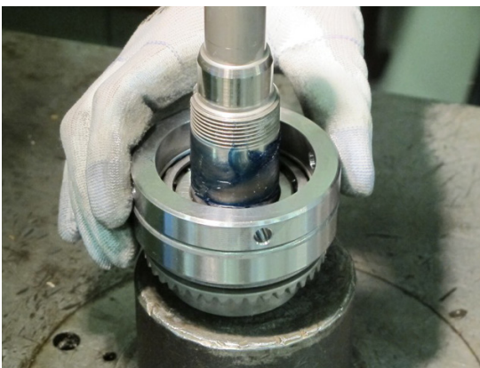
3. Place the distance ring on the big tapered roller bearing.
