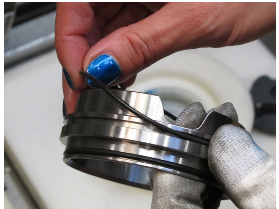
11. Assemble the O-rings on the distance ring.
