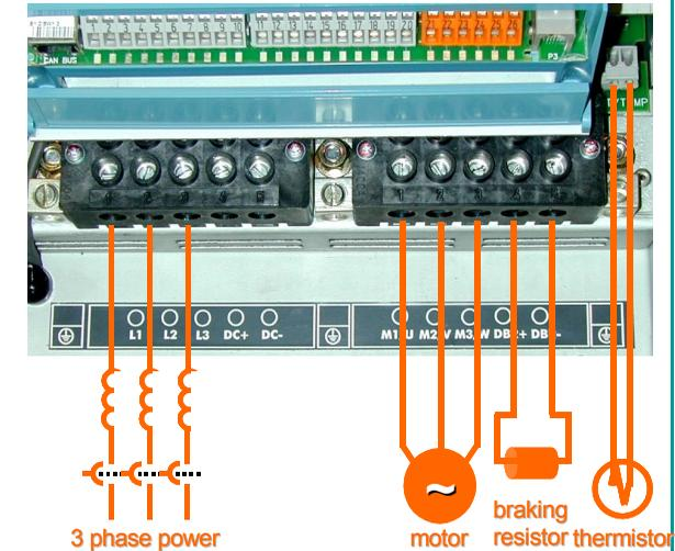
The power terminals shown are for frame D. Although other frames may vary slightly in appearance, their terminal designations and functionality are identical
