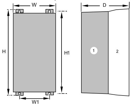
(1): Electronics (2): Head dissipator
