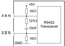
The input connection is available in triple (for A & /A, B & /B, N & /N)
